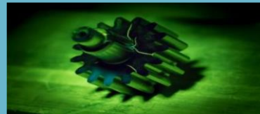
Notched Shim (also called quantitative quality indicator, or QQI)
